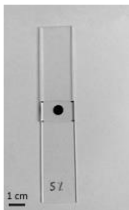
Figure S 6: Photo of a lap shear test sample.
