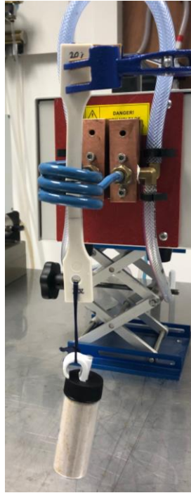
Figure 5: Image showing the sample setting for the OMF initiated debonding experiments.
