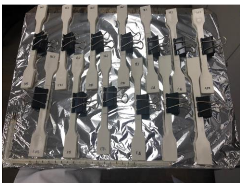
Figure S 8: Photo of dog-bone shaped samples for debonding experiment under OMF condition prior to heating in and oven.
