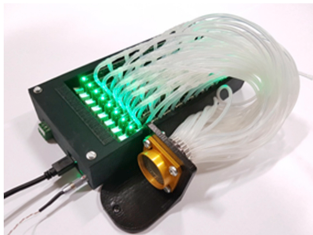
Fig. 11. Overview of the 64-channel pressure tapping system used during this work.
