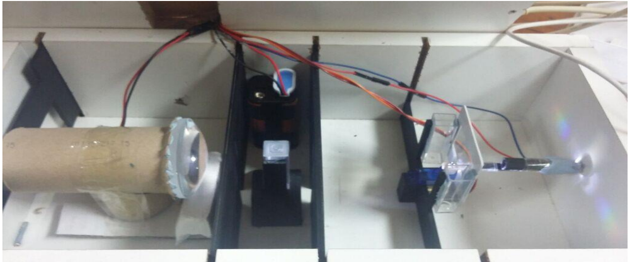
Figure 1. UV spectrometer built in 2015/16.
