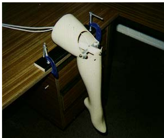
Figure 4. The artificial leg, showing hinge mechanism and entry point
