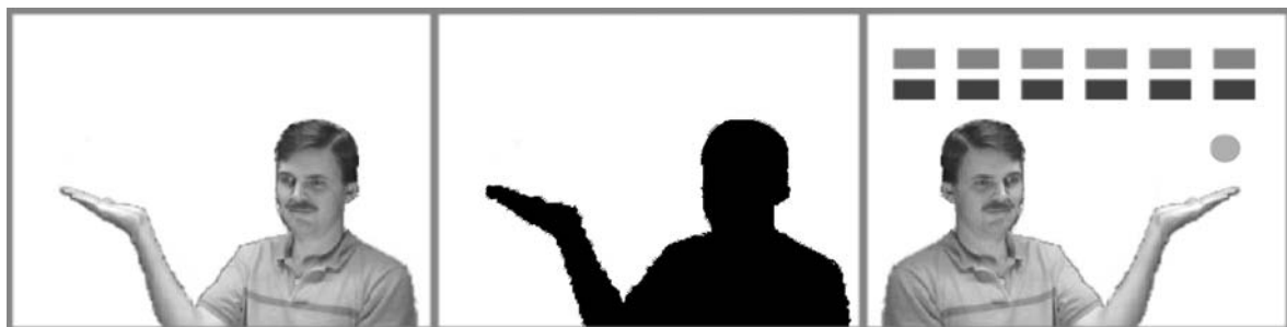
Figure 3. Example images at various points in the Virtual Interaction system. The left image is typical of the camera output. The center image is the user's silhouette, as produced by the chromakey. This is the image that the system reacts to. The image on the right is the resulting image shown to the user.
