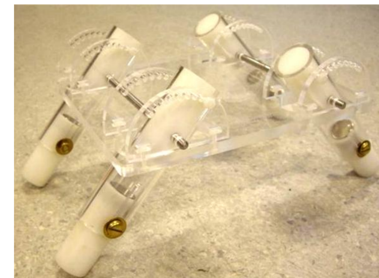
Figure 4: DMCU Robot Test Rig with 4 DMCU modules
