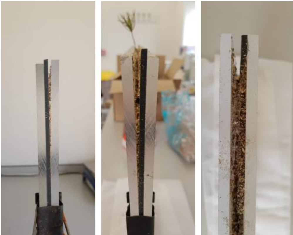
Figure 3.6. Gaps opened in the microcosms due to the folding back of the Perspex plates. In some cases, the gaps between the plates were as wide as 0.5 cm.
