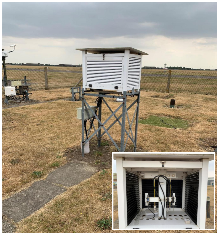
Figure 9. General view of the site at Coningsby, and (inset) detail of the screen interior; both photographs were taken on 20 July 2022. (Source: Met Office SWAT report: ©Crown.)
