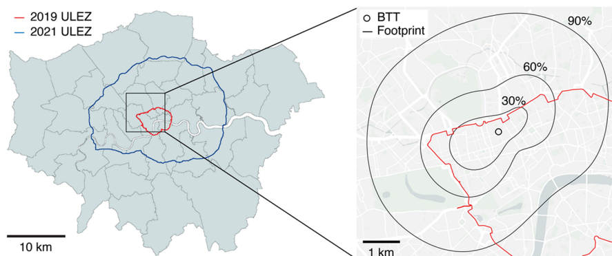
Figure 1. Average measurement footprint for the BT Tower (BTT) displayed as a series of contours, each of which represents a percentage of the contribution. Footprint is shown relative to the Greater London area and the locations of the ultralow emissions zone (ULEZ) boundaries. Map data courtesy of OpenStreetMap contributors, distributed under the Open Data Commons Open Database License v1.0.
