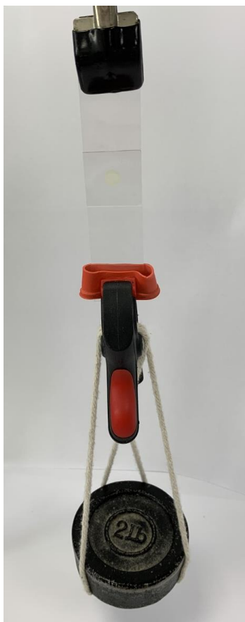
Figure 155. An image of a 7 mm diameter sample of SPU12 adhered between 2 glass slides holding a 2 lb (0.907 Kg) weight.
