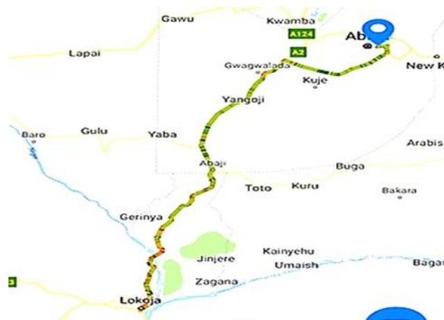
Figure 2: Screenshot of IRI measurement for road link (RoadLab Pro)
