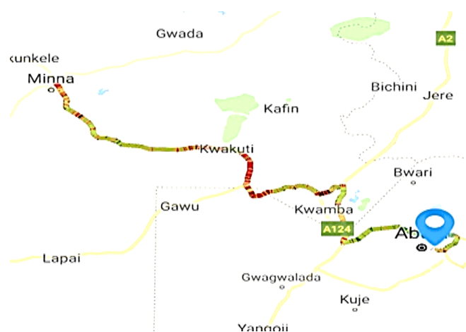
Figure 1: Screenshot of IRI measurement for road link (RoadLab Pro)
