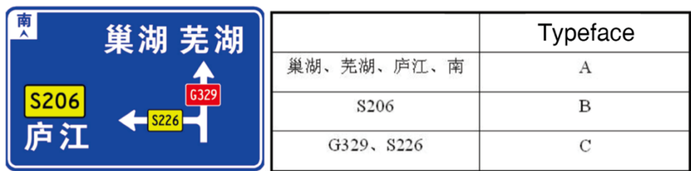
Figure 3-3. The illustration of applying the three typefaces to a Chinese traffic sign. Typeface B is used for the route number, exit number, and kilometers; Typeface C is used for the route number placed on the route arm; Typeface A is used for the rest of the situations. Extracted from Standard f., 2017, page 11.
