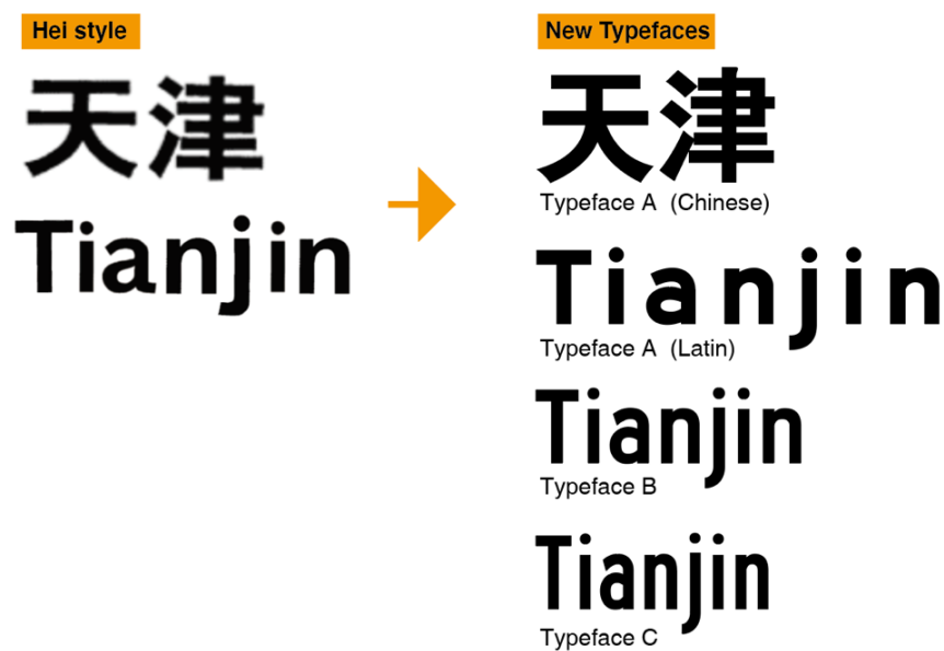
Figure 3-3. The illustration of applying the three typefaces to a Chinese traffic sign. Typeface B is used for the route number, exit number, and kilometers; Typeface C is used for the route number placed on the route arm; Typeface A is used for the rest of the situations. Extracted from Standard f., 2017, page 11.
