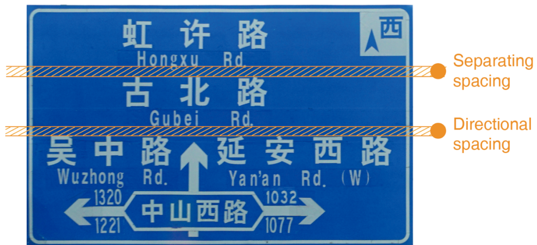
Figure 6-12. Separating spacing and directional spacing on a three-direction sign. Illustrated by the author. Photographed by author, Shanghai, 2018.
