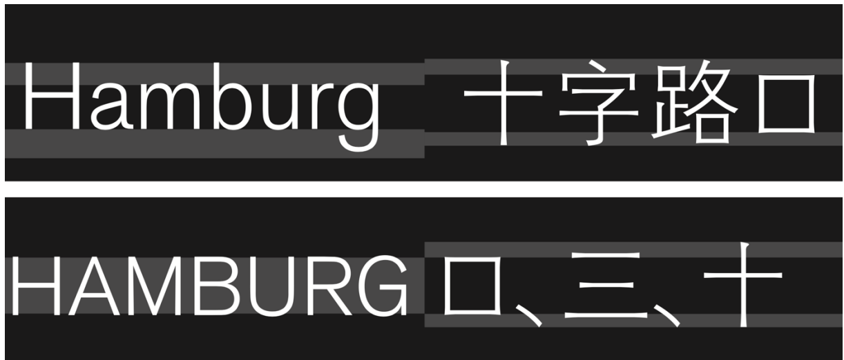
Figure 1-3. Optical guides in both Latin and Chinese typeface. Latin typefaces crucially stick to the baseline, as well as to the x-height and Chinese typefaces stick to the optical centre line. Based on this, to achieve an optical harmonious match, Roman Wilhelm provides some approaches. 'Typed upper and lower case, Latin characters range between ascender, descender, caps height, x-height and baseline. This provides a dynamic feeling which can be able to match with Chinese characters ranging between '十-height' and '口-height'. Typed upper case, the impression changes to rather static. In many cases, the '口-height' may help adjusting, as well as the '三' character.'
