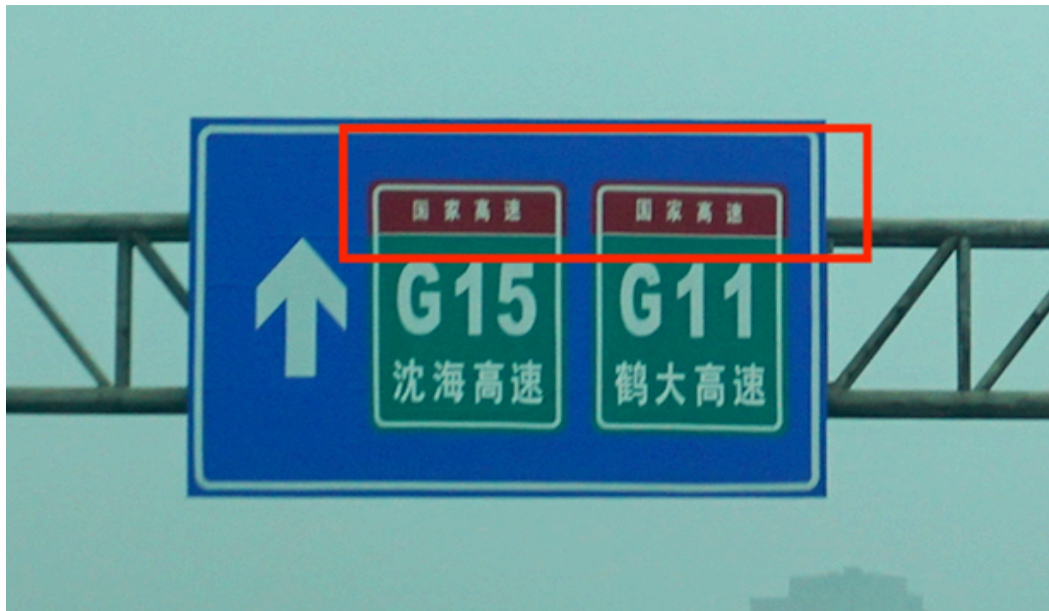
Figure 4-2. Standard guidelines fail to meet practical needs. The design of the four white Chinese characters ‘国家高速’ (marked in a red rectangle) meet the Standard specifications, but they can hardly be read in practice because of the small type size. This photo supports Implementor ’s opinion that the guidance, sometimes, cannot meet practice needs. Photographed by the author, Dalian, 2018.
