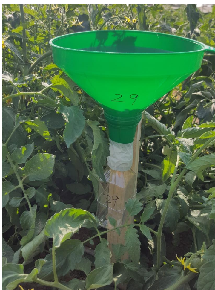
Figure 4.3 Funnel (20cm diameter) connected to a 300ml transparent plastic bottle to collect the pesticide deposition.
