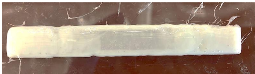
Figure 4.3.5: Picture of a printed MGP bar semi-automatically.
