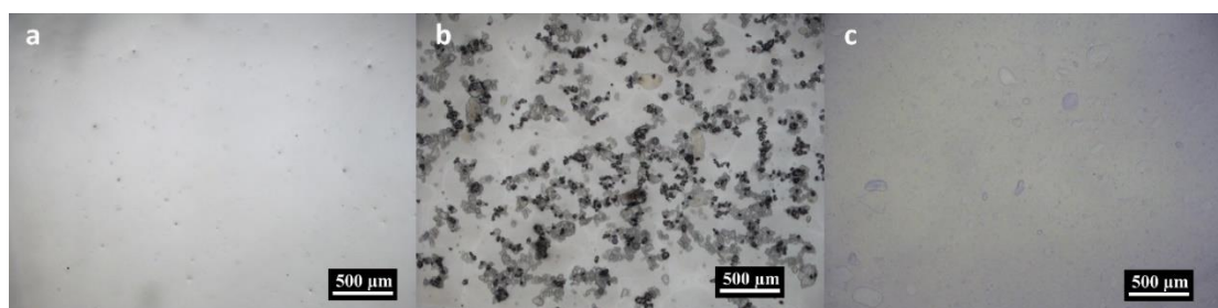
Figure 5.3.19: Optical microscopic images of the polyol inks with the formulation presented in Table 5.3.8 a) PDMS-SiNP , b) H 2 N-SiNP and c) NH 2 /CH 3 -SiNP-03 .
