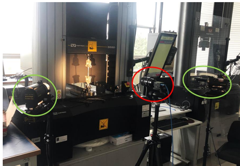
Figure 4.3.9: Image of the DIC experiment setting. The camera in the middle defined by red circle and two spotlights determined by green circles.
