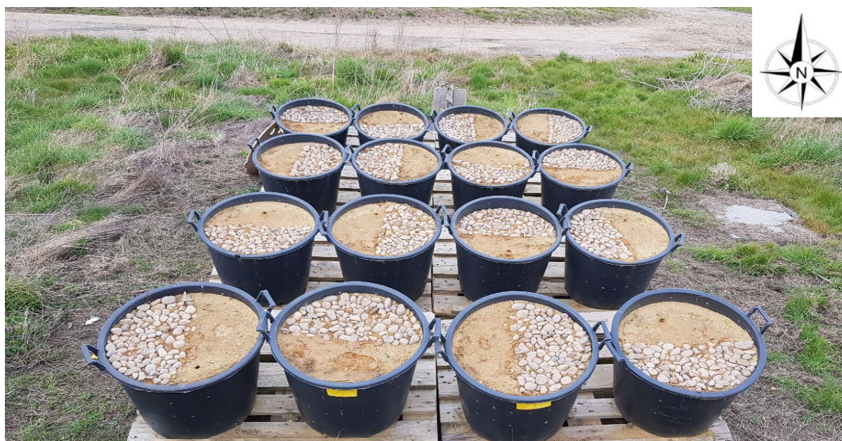
Figure 4.4: Soil compaction trial with pebble and bare soil treatments in each block.
