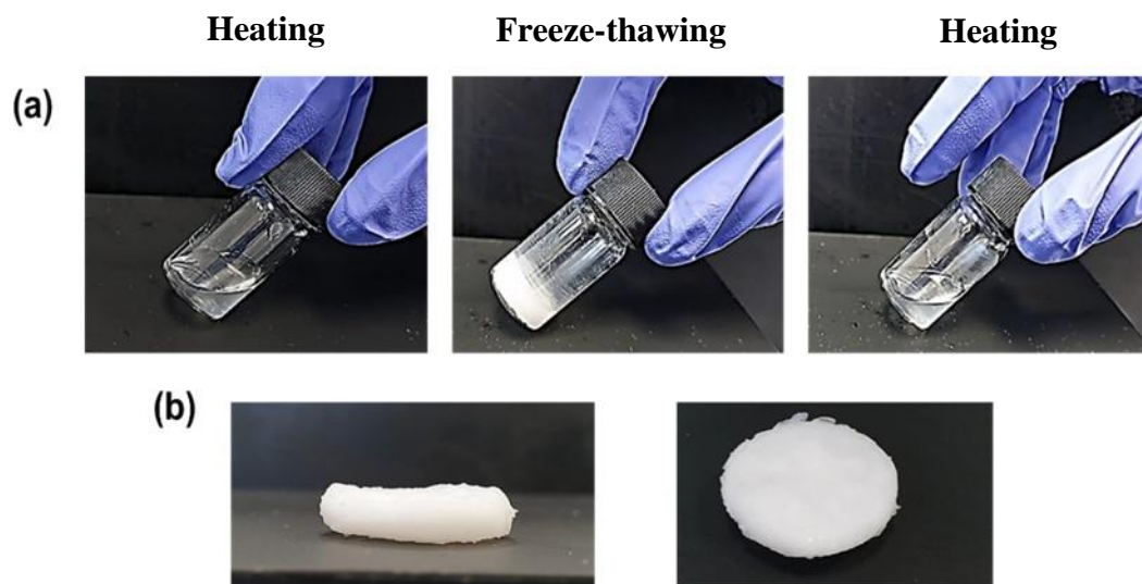
Fig. 11. Solution – gel – solution transition of L-PEI cryogels. The solution is initially heated to 80 °C forming a transparent solution. After freezing at - 80 °C for 3 h and then thawing at room temperature, an opaque gel is produced which, on subsequent heating to 80 °C, returns to a transparent solution (a). Appearance of L-PEI cryogels (b) [29].
