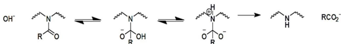
Fig. 5. Schematic diagram of basic hydrolysis of PEOZ to form linear PEI [15].
