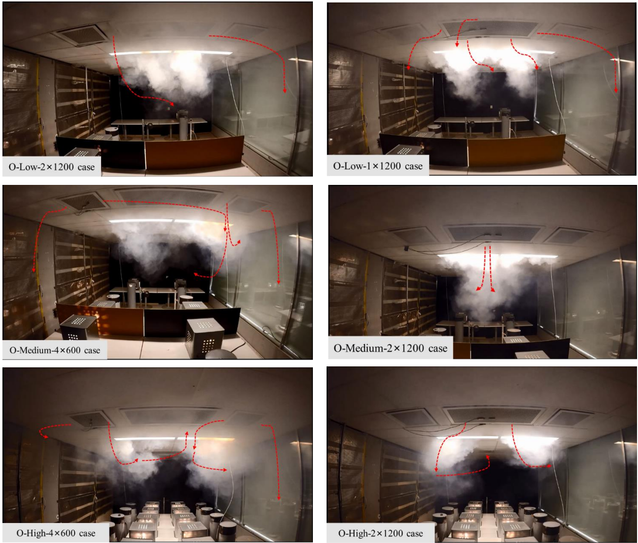
Fig. 5: The visualized airflow patterns under different heat gains and different chilled beam types. (Note: Red arrows depict the direction of the supply air in those conditions.)
