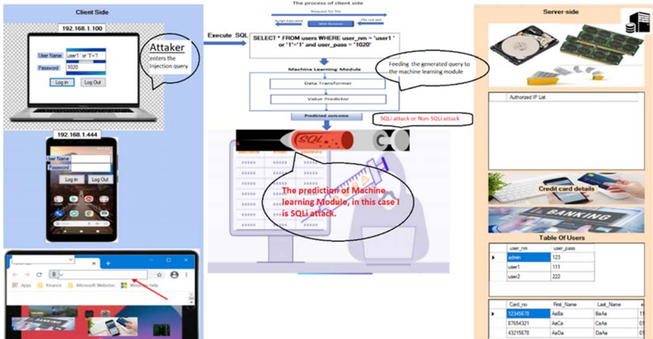
Fig. 11 ML algorithm has recognised the Injection query
