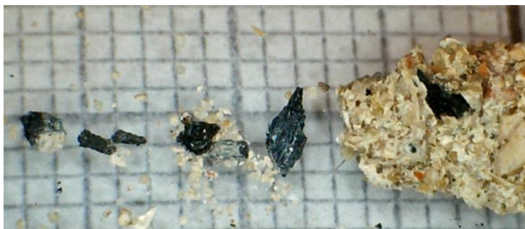
Fig. 4. Lyminge Church mortar Sample 1 (Large block) charcoal (divisions 1mm)
